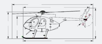
Ground to Rotor Height8.65 ft. (2.64 m)Ground to Fuselage Bottom Height1.77 ft. (0.54 m)Main Rotor Diameter27.50 ft. (8.38 m)Tail Rotor Diameter5.08 ft. (1.55 m)
